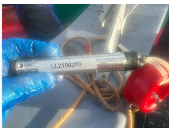
Solinst Levellogger and Hobo MX2200 Pendant instruments as deployed (Locations 4cA and 3b respectively)
